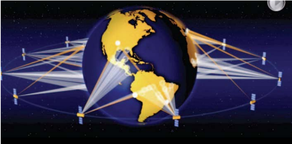
Figure 3 shows the MEO satellite constellation coverage area from an Equatorial orbit
